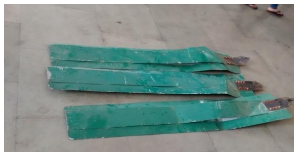
Figure.4 Damaged Blades Due To Designing Error
